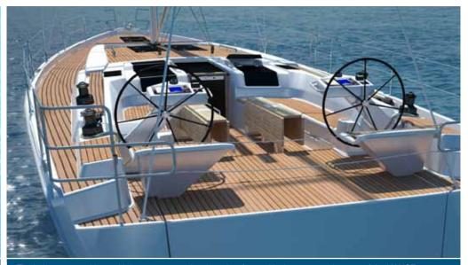
The helmsman positions with luxury seats and a clear view forward is the command center of the HANSE 575. All halyards, sheets and trimming lines are easy to handle from here. Thanks to the self tacking jib crew assistance is not needed for every manoeuvre. Just sail and relax.
